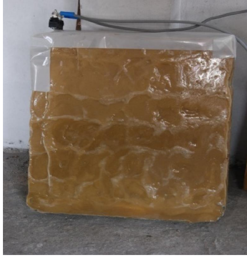
Figure 13: 12.24 mF, 45 A low voltage AC capacitor specifically developed for experimental verification and as required by the filter design
